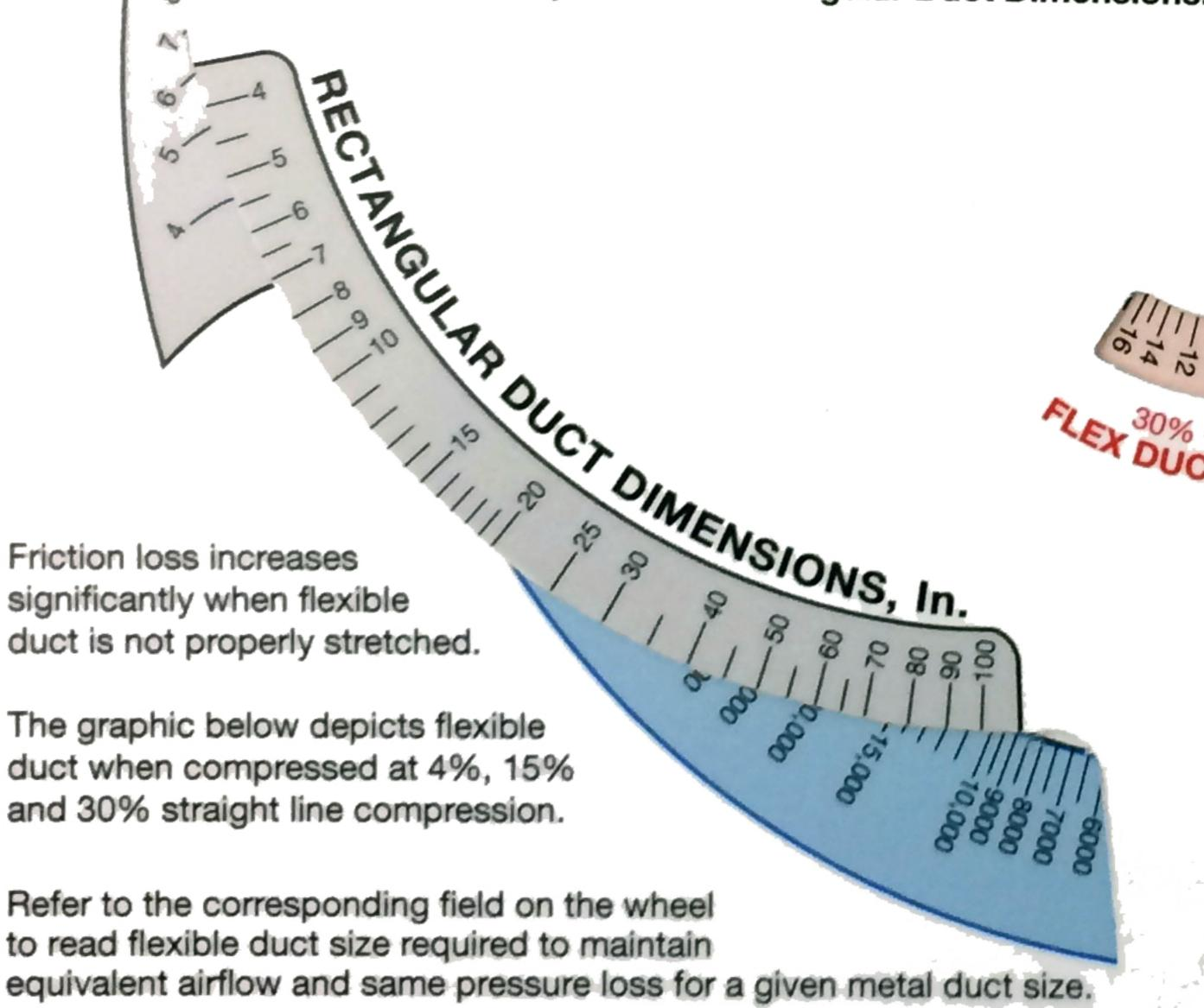
Note: Bends, curves and excessive lengths in flexible duct will add additional friction losses.
