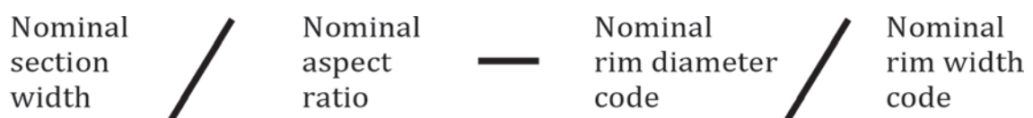
Figure 1 — — Indication of dimensional and constructional characteristics
