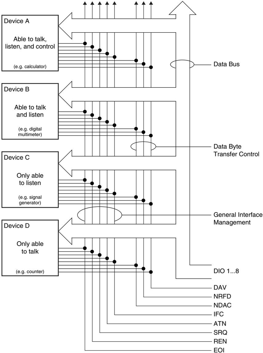
Figure 1—Interface capabilities and bus structure
