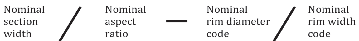
Figure 1 — — Indication of dimensional and constructional characteristics
